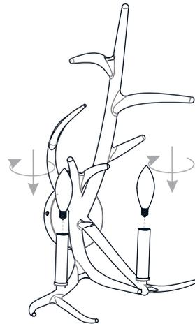
Install two correct bulbs referring to fixture markings and/or labels for maximum wattage.
